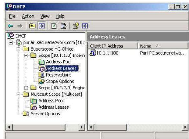
addresses to DHCP clients, and with no manual intervention. IP addresses that are assigned via a DHCP server are regarded as *dynamically assigned IP addresses*. The DHCP server assigns IP addresses from a predetermined IP address range(s), called a scope.
