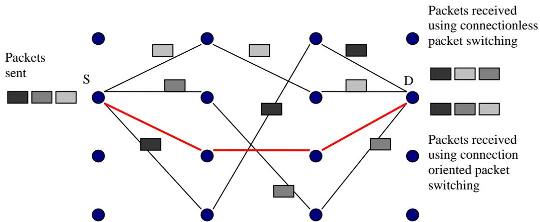
Fig. L 4.1 Connectionless and connection oriented packet switching
