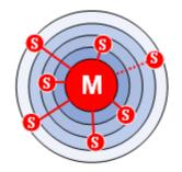
In reality, at a given moment, the master device can only be connected to a single slave at once. Therefore, it quickly switches between slaves in order to make it seem as if it is simultaneously connected to all the slave devices.
