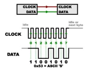
One reason that SPI is so popular is that the receiving hardware can be a simple shift register. This is a much simpler (and cheaper!) piece of hardware than the full-up UART (Universal Asynchronous Receiver / Transmitter) that asynchronous serial requires.
