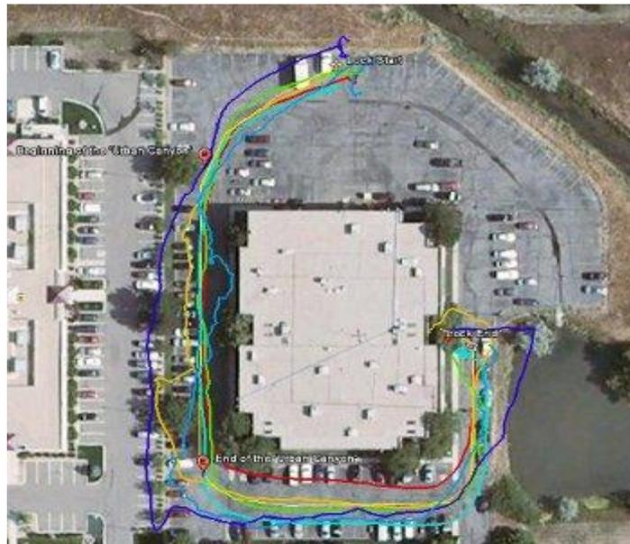
*Logged and plotted GPS waypoints around SparkFun headquarters. Each track represents a different type of GPS module.*
