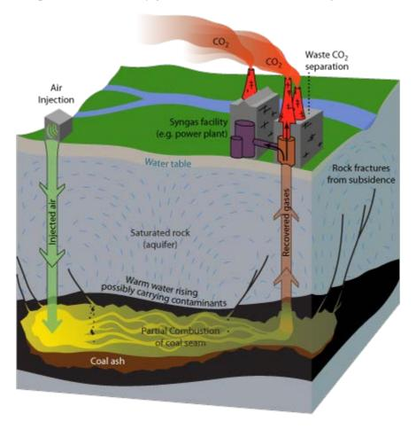
*Underground Coal Gasification:* Underground Coal Gasification involves igniting a coal seam underground and pumping out the partially burned gases that result.
