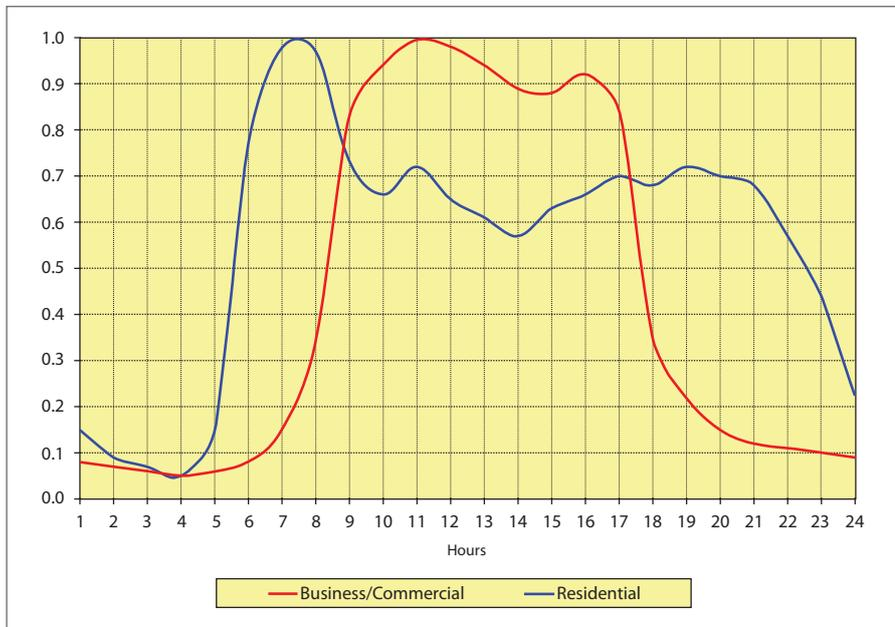
Figure 1: Typical unit hydrographs for sewer flows
