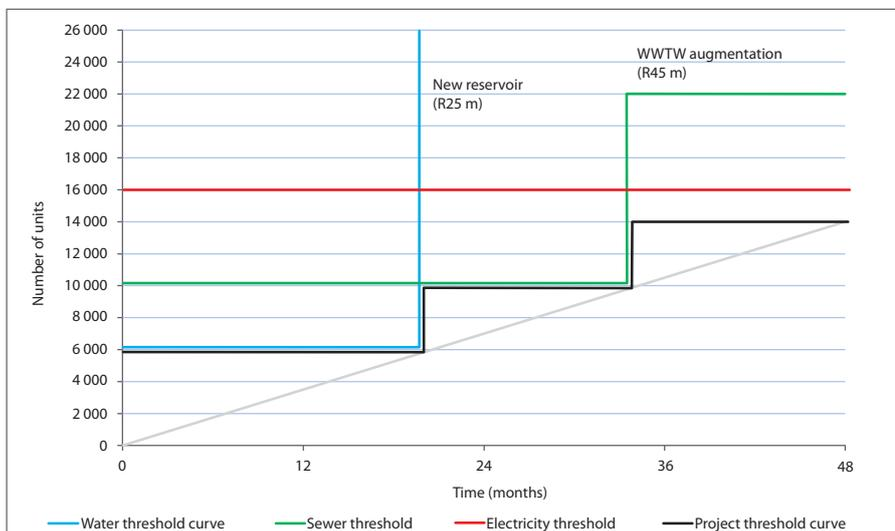
Figure 2: Infrastructure threshold curve for the development of 14 000 units
