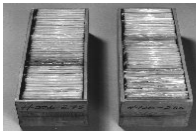
Figure 2 a: An example of damage spreading from a point source of corrosive vapour. The two boxes each contain around 1500 nitrate negatives. The dark spots are caused by deteriorating film base.
