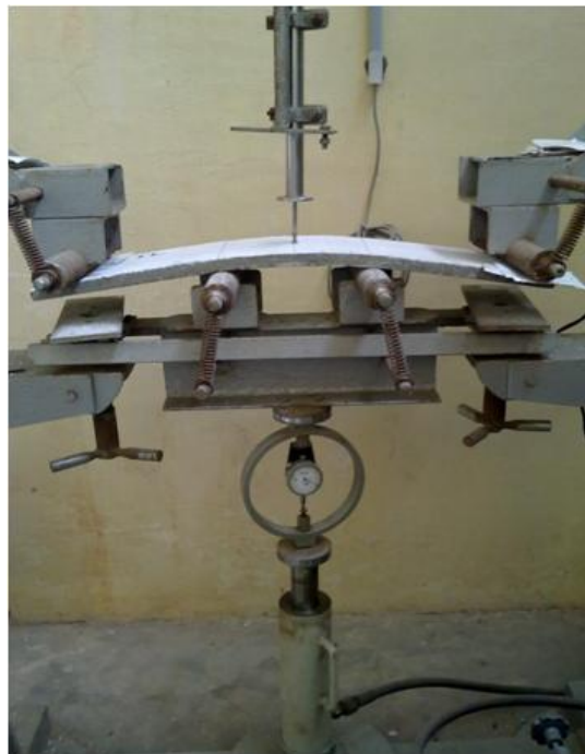
Fig. 5 Ductility of Ferrocement Slabs
