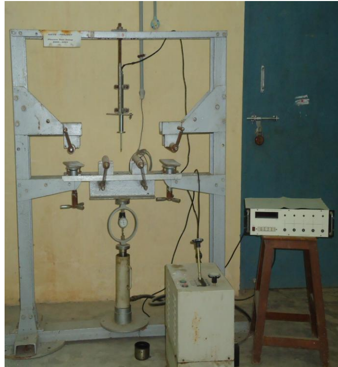
Fig. 2 Flexure Test Set-up
