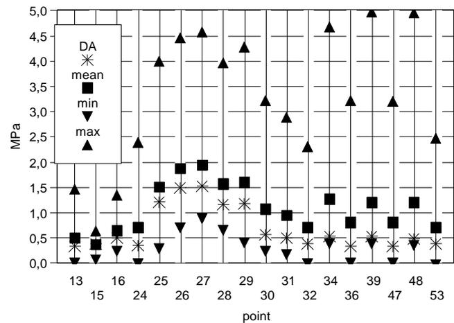
Fig. 3 Principal stress  $\sigma_1$  in points on lower surface
