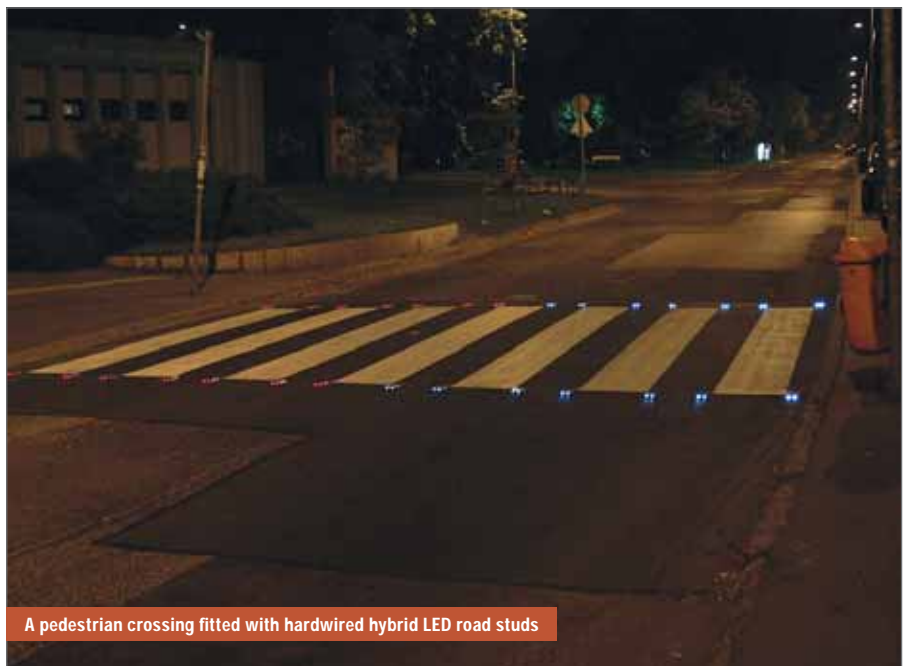
The hardwired LED stud is a 24-hour operational road stud for use at pedestrian crossings, speed bumps and intersections
