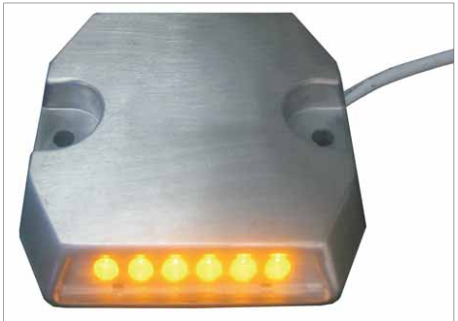
The hardwired LED stud is a 24-hour operational road stud for use at pedestrian crossings, speed bumps and intersections
