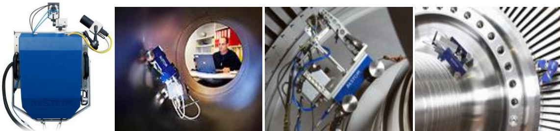
Fig. 7 The AIR service modular robot in the control process of an impeller [14]
