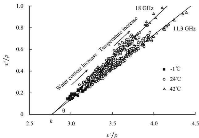
Figure 6 Complex-plane plot of the dielectric constants and loss factors, divided by bulk density,  $\rho$ , of hard red winter wheat of various moisture contents and bulk densities at indicated temperatures for two frequencies, 11.3 and 18.0 GHz<sup>[40]</sup>.
