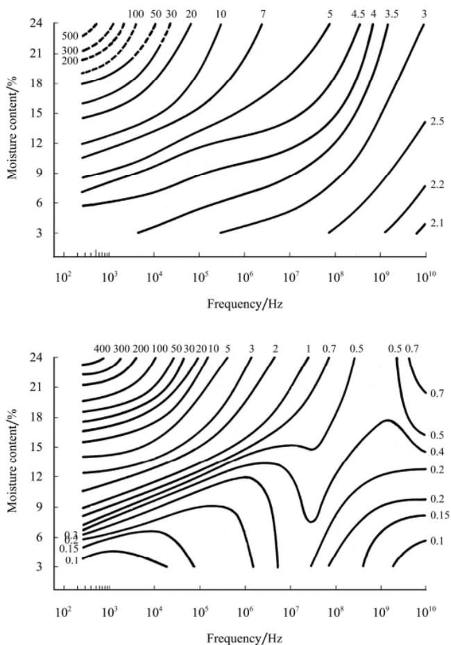
Figure 3 Dielectric constants,  $\epsilon'$ , and loss factors,  $\epsilon''$ , for hard red winter wheat at 24°C at frequencies from 25 Hz to 10 GHz and moisture contents from 3% to 24% at natural densities. Mean values for seven cultivars<sup>[11,12]</sup>
