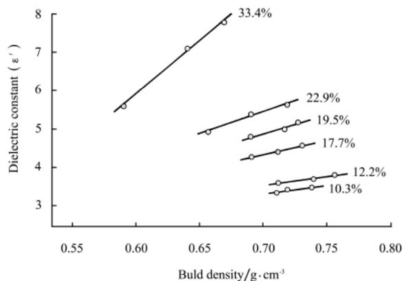
Figure 5 Density dependence of the dielectric constant of shelled yellow-dent field corn at 24 °C, 20 MHz, and indicated moisture contents<sup>[13]</sup>
