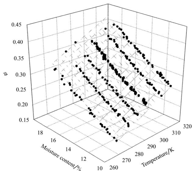
Figure 7 Moisture and temperature dependence of density-independent moisture calibration function  $\psi$  at 14.2 GHz for hard red winter wheat<sup>[45]</sup>.
