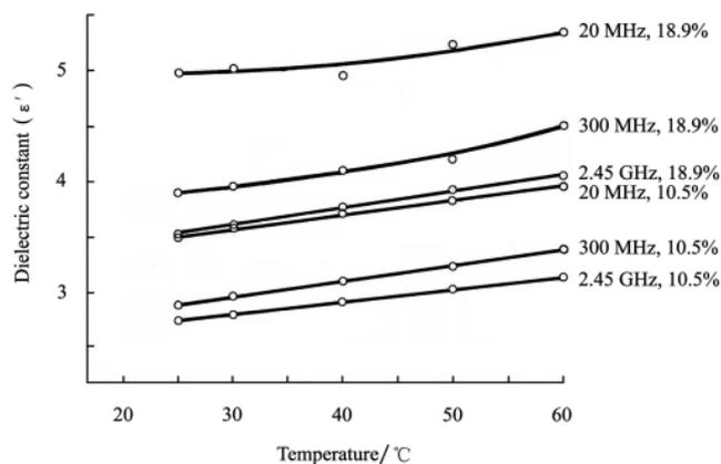
Figure 4 Temperature dependence of the dielectric constants,  $\epsilon'$ , of shelled yellow-dent field corn at indicated frequencies and moisture contents<sup>[24]</sup>.
