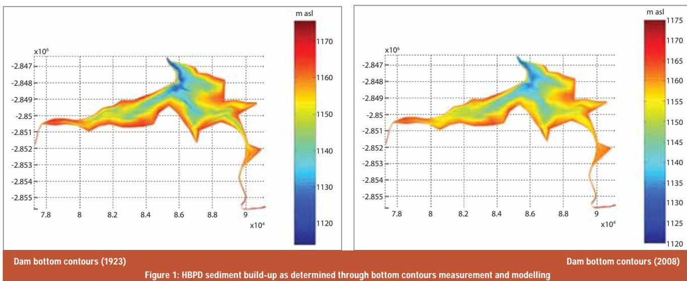
Figure 1: HBPD sediment build-up as determined through bottom contours measurement and modelling
