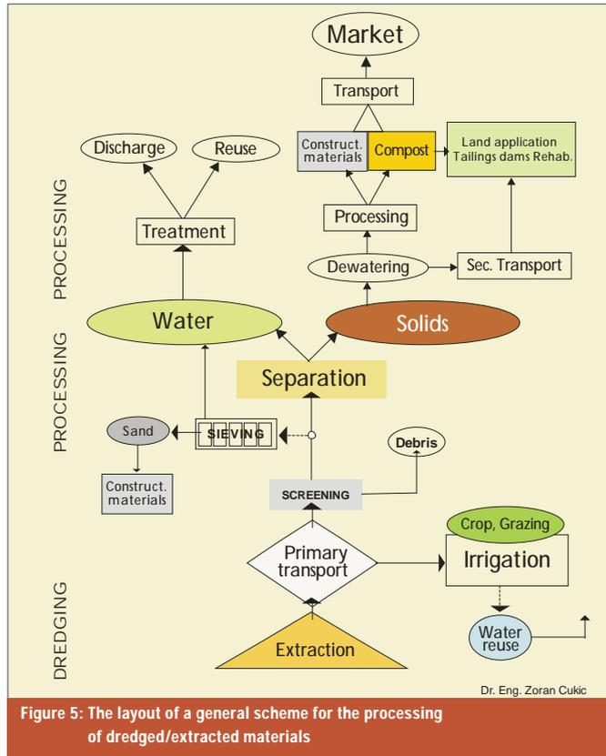
Figure 5: The layout of a general scheme for the processing of dredged/extracted materials
