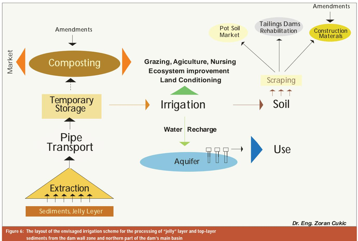
Figure 6: The layout of the envisaged irrigation scheme for the processing of "jelly" layer and top-layer sediments from the dam wall zone and northern part of the dam's main basin
