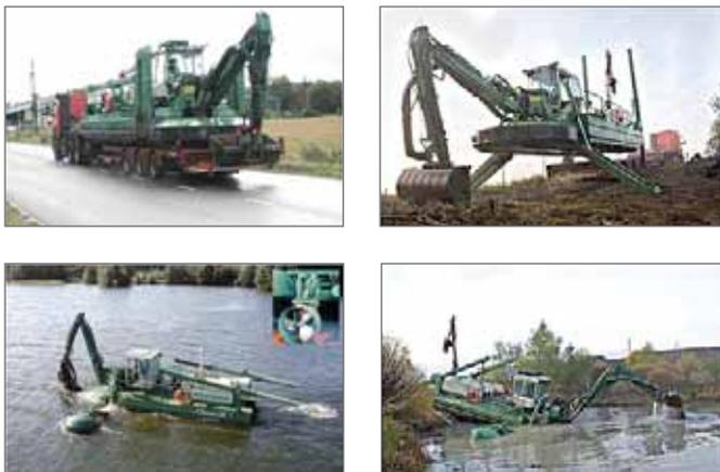
Figure 4: Mobile, multi-purpose, shallow-water dredging equipment (to be purchased)
