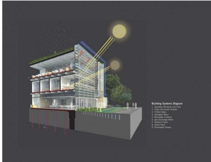
But by utilizing an array of sensors and systems this modern building is capable of monitoring and measuring its energy and water use in real-time. Depending on the environmental conditions, the building can automatically alter external shades to help cool or heat the building via sunlight, reducing the need to use energy, and allowing it to keep running at its greenest possible performance.
