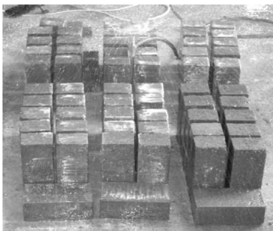
Fig.3 The curing of paving block samples
