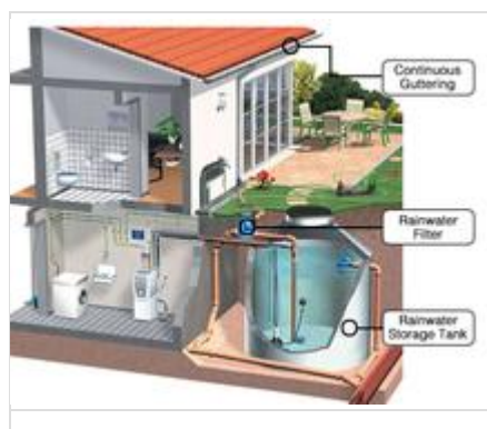
Figure 4: Complex RWH system with filtration
