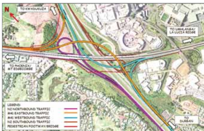
Figure 1: The upgraded Mount Edgecombe Interchange configuration
