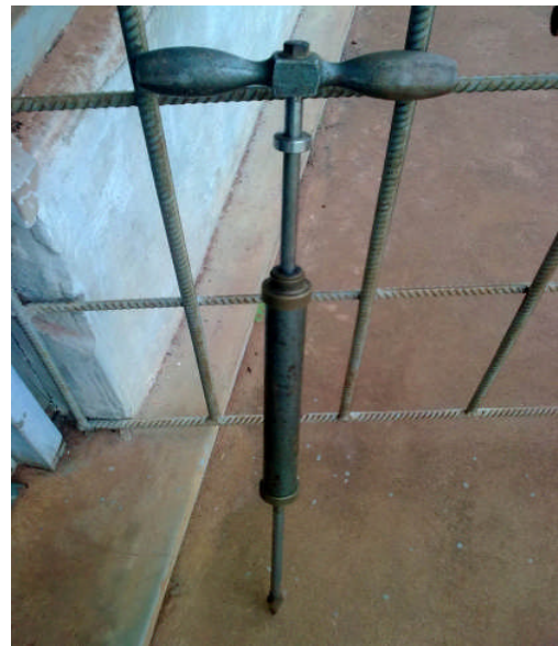
Figure 6 Imported proctor-type penetrometer
