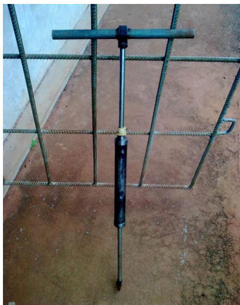
Figure 5 Locally produced proctor-type penetrometer
