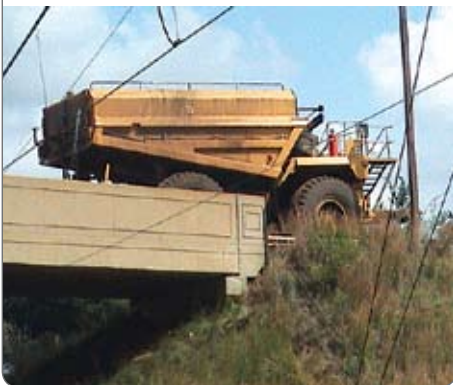
Figure 4 Full-scale load test in progress
