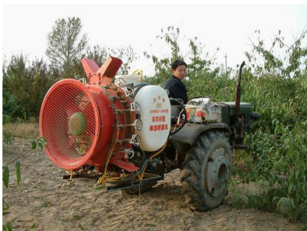
Figure 3 Photo of the automatic target detecting orchard sprayer working in orchard
