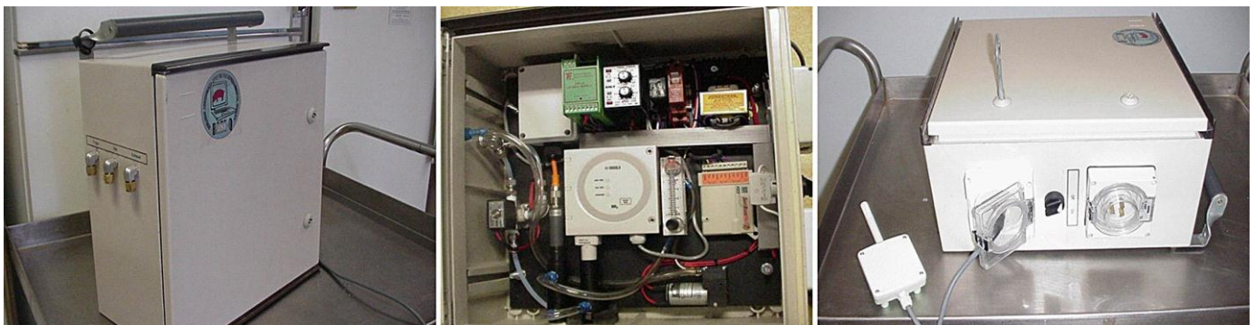
Figure 5 Environmental monitoring modules of the BASE-Q system [24]
