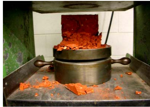
Fig. 6 Compressive strength test
