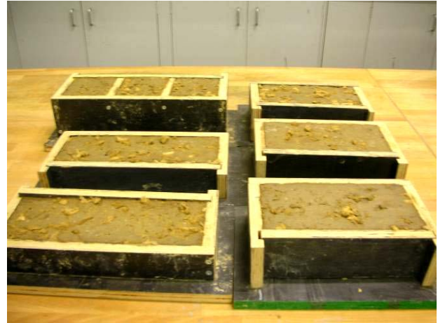
Fig. 2 Compacted bricks, beams and cubes (soil-CBs mix)
