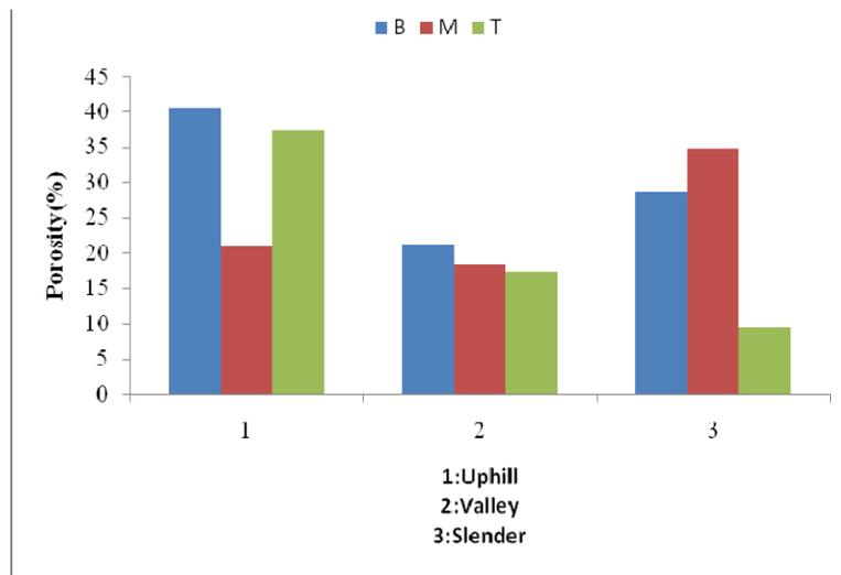
Figure 10 : Effects of tree origin and the position on a tree on the porosity of bamboo with node
