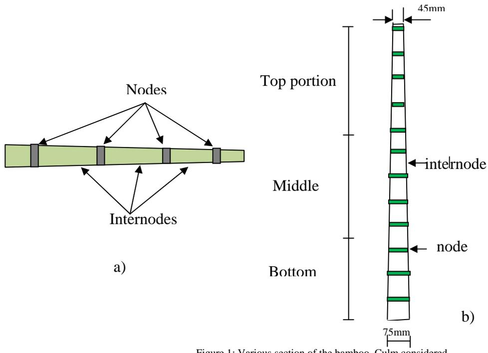
Figure 1: Various section of the bamboo Culm considered
