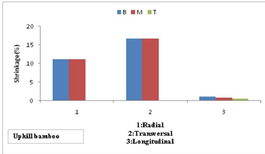
Figure 11 : Variation of the shrinkage for various direction in the tree for uphill bamboo
