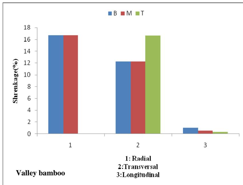
Figure 12 : Variation of the shrinkage for various direction in the tree for valley bamboo
