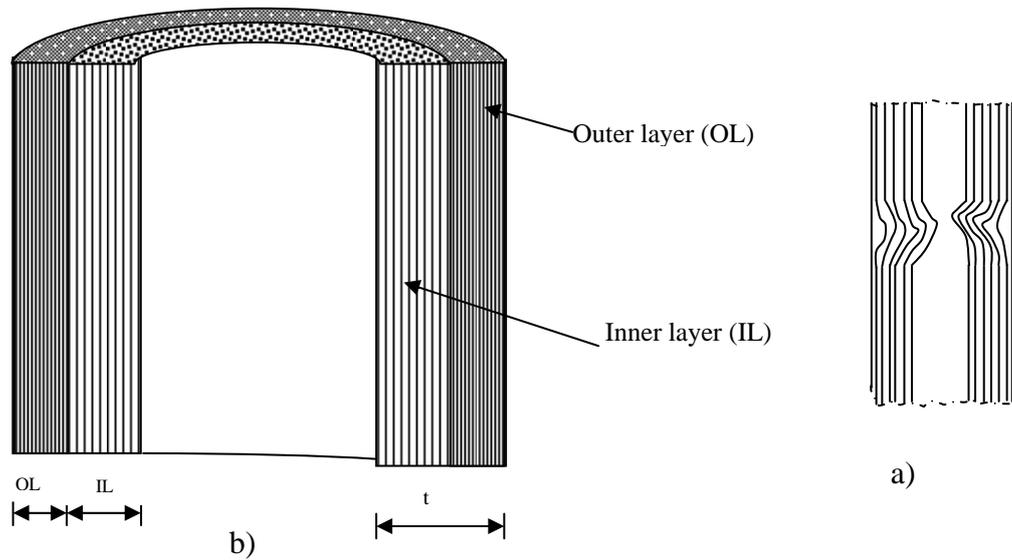
Figure 2: Various layer of the bamboo culm and configuration of fibres for the inner and outer layers
