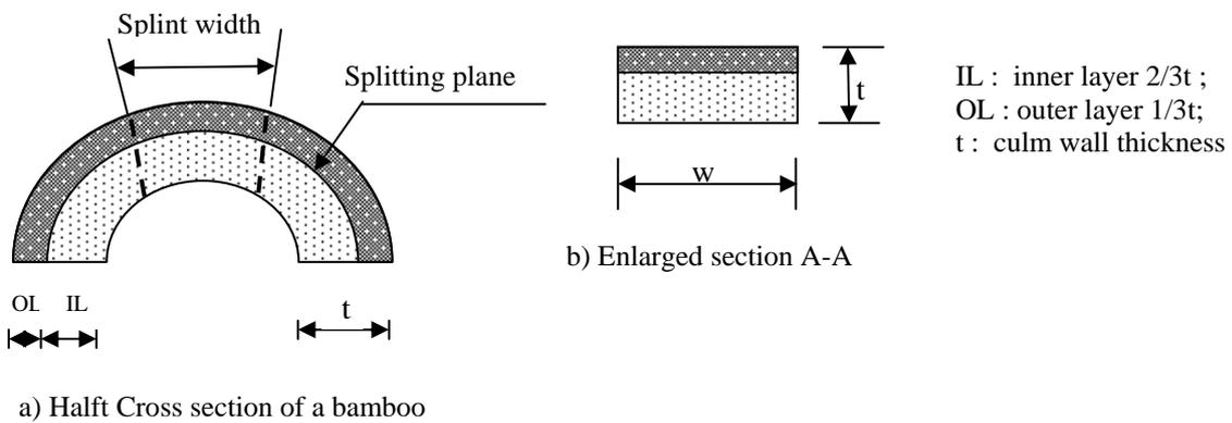
Figure 3 : Definition of the split for the test
