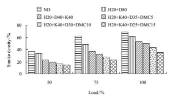
Figure 6 Variation of smoke density with load
