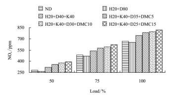
Figure 7 Variation of NO<sub>x</sub> with load
