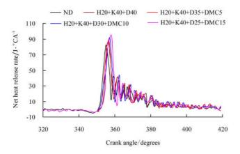
Figure 10 Net heat release rate with crank angle
