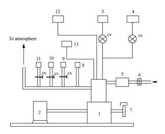
1. Engine 2. Eddycurent dynamometer 3. Diesel tank 4. Honne oil tank 5. Air tank 6. Orifice meter 7. Speed pick up 8. EGT, 9. Smoke meter 10. Exhaust gas analyzer 11.  $SO_2$  meter 12. Computer, display unit (PV, P0, NHRR etc) 13. Lubricating oil temperature, CV = control valvel
