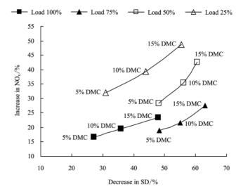
Figure 8 Trade off between SD and NO<sub>x</sub>
