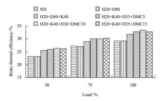
Figure 3 Variation of brake thermal efficiency
