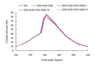
Figure 9 Cylinder pressure with crank angle
