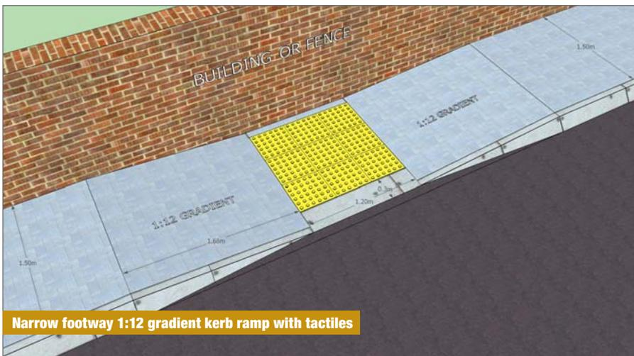
**Narrow footway 1:12 gradient kerb ramp with tactiles**
