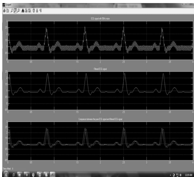
Fig. 4 The 50Hz noise filtered from ECG signal using nyquist filter designed by Kaiser Window (ECG signal with 50 Hz noise, filtered signal, comparison between the pure ECG signal and filtered signal)
