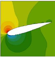
b. Iced blade (  $\alpha = 15^{\circ}$ , U=8 m/s, Q=0.5 L/min)
