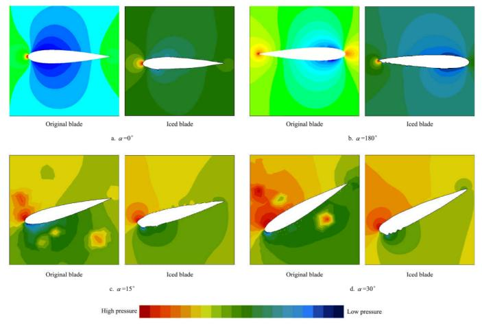
Figure 5 Pressure contours for the original blade and iced blade at different attack angles
