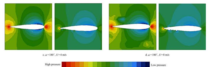
Figure 6 Pressure contours for the original blade and iced blade at different wind speeds
