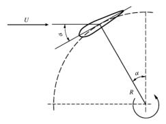
Figure 4 Definition of the attack angle of the blade
