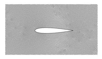
Figure 3 Grid mesh around the blade
