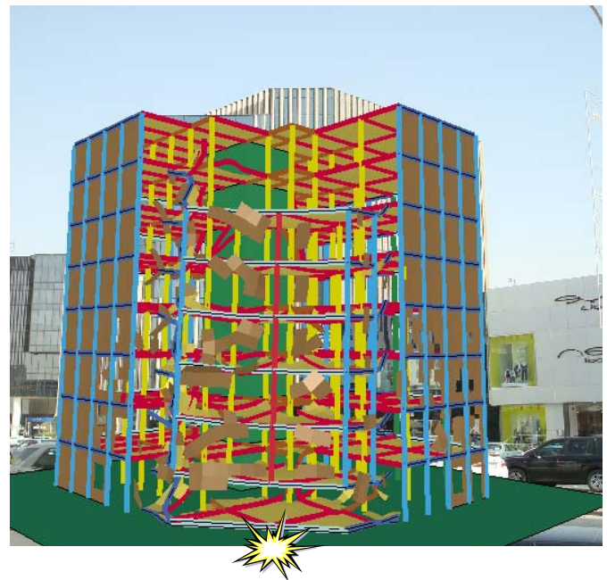
Fig. 9 Partial collapse of the building at 6s
