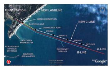
Layout of marine outfall systems A-, B- and C-line
