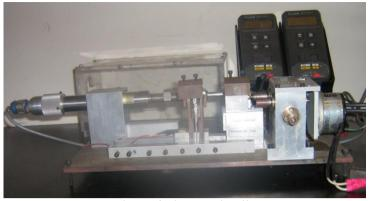
Figure 4 Fibre testing jig
