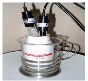
FIG 3: Potassium Sensor electrode and reference electrode are immersed in 10<sup>-3</sup> M buffer solution
