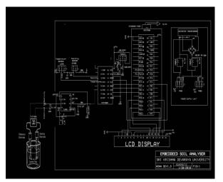
Fig.4: Schematic Diagram of Embedded Soil Analyzer
