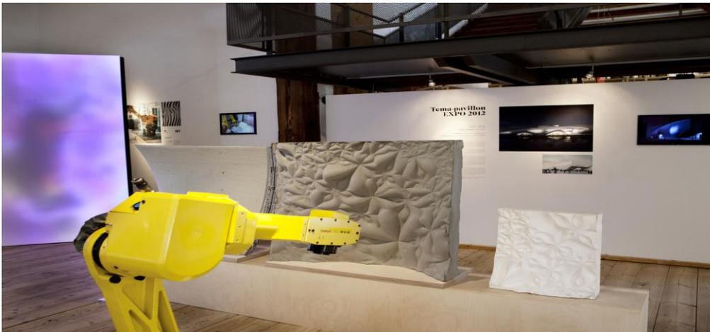
Also exhibited is a machine which sculpts concrete, a 3D façades` printer. Tailor Crete undertakes infinite design patterns, saves time and is praised for its effectiveness and detailed work quality.
