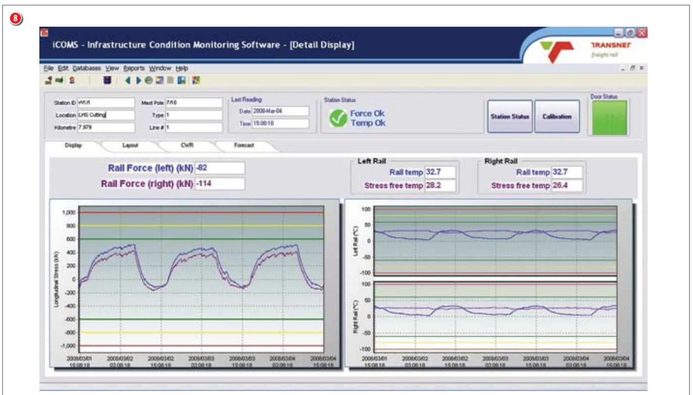
8 Example of longitudinal rail force data
