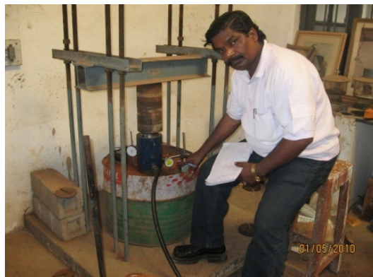
Fig. 9: Author is conducting the Static Plate Load test
