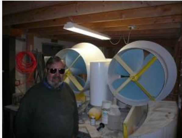
Models of kinetic power generator for tidal currents; similar to the CleanCurrent design used in BC (photo by toddraden @flickr--click on image for source)
