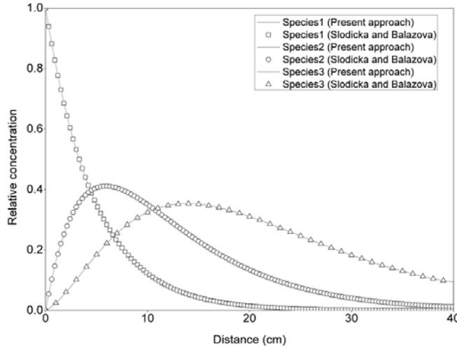
Figure 3. Comparison of the finite difference solution for three species reactive transport system with that of Slodicka and Balazova (2009).
