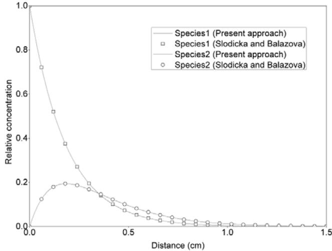
Figure 1. Comparison of the finite difference solution for identical reaction rates with that of Slodicka and Balazova (2009).
