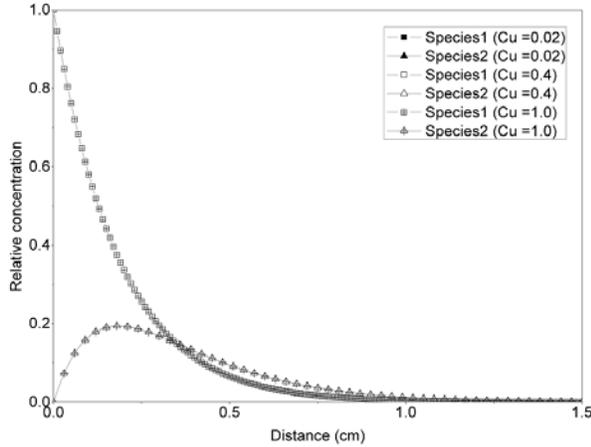
Figure 2. Spatial distribution of concentration obtained from the finite difference model for different Courant numbers.
