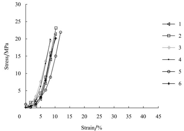
Figure 4 Reed compressed stress-strain multinomial drafted curve
