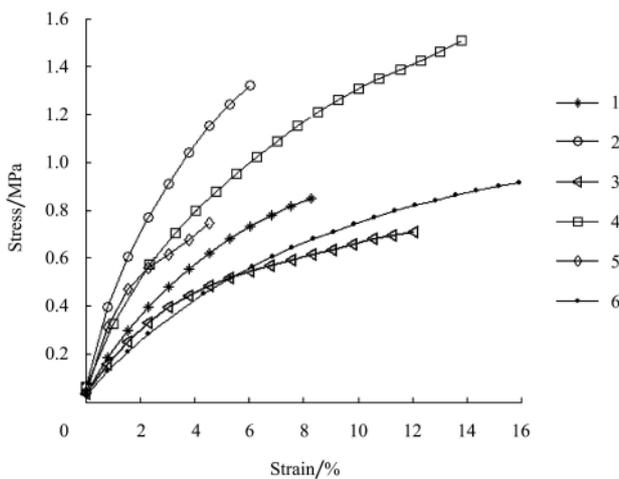
Figure 8 Reed bending stress-strain multinomial drafted curve
