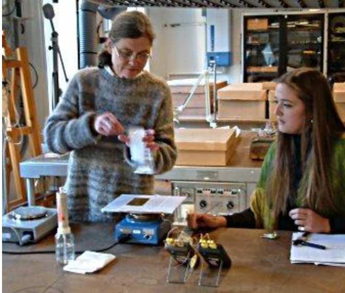
Kaisa (left) has just removed the damp cloth specimen from the warm plate and is putting it into a zip-lock PE bag for weighing. Henrietta notes the temperature of the cloth surface, using the two thermocouple digital thermometers in the foreground.
