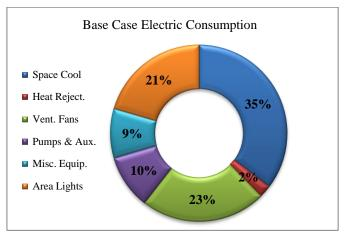
Figure 4: Base case energy consumption breakdown in percentage
