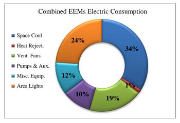
Figure 5: Combined EEMs energy consumption breakdown in percentage
