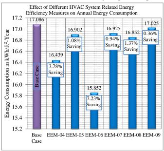
Figure 8: Effect of Different HVAC System Related EEMs on Annual Energy Consumption
