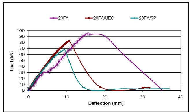
Fig. 12 Load deflection curves of 20% fly ash concrete beams
