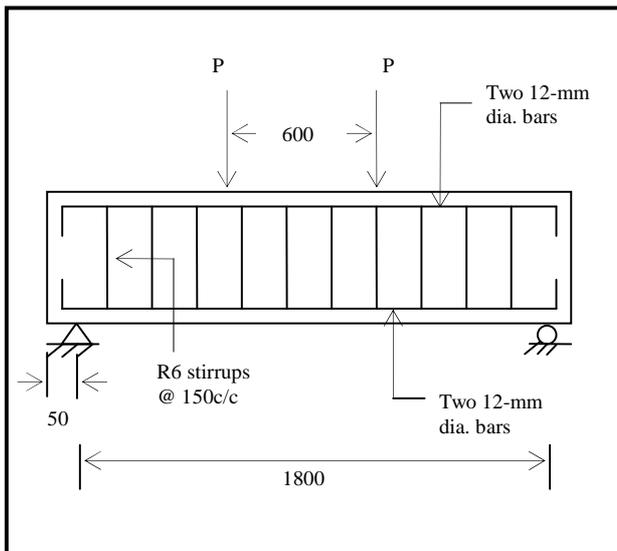
Fig. 1 Details of test specimen (unit in mm)
