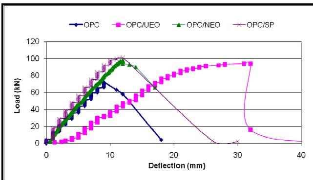
Fig. 11 Load deflection curves of 100% OPC concrete beams
