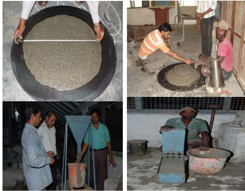
Fig: 1. workability test on the SCC
