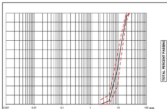
Fig. 1 Curve of coarse aggregates grading
