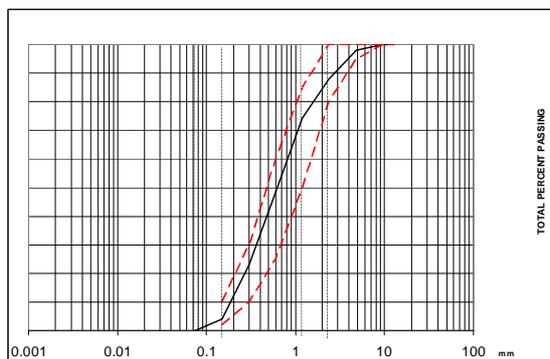
Fig. 2 Curve of fine aggregate grading
