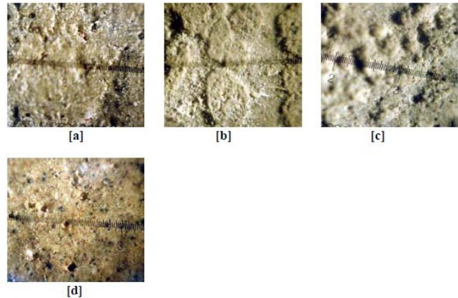
Fig. 3 Surface image of GP8.5 specimen at different temperatures as seen through optical microscope
