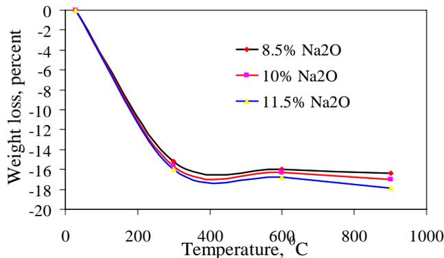
Fig. 11 Weight loss of geopolymer specimen with temperature
