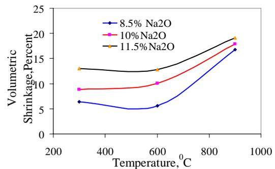
Fig. 10 Variation of volumetric shrinkage of geopolymer specimen with temperature
