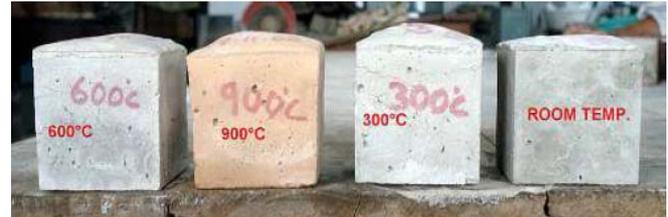
Fig. 2 Photograph of GP8.5 specimen at different temperatures
