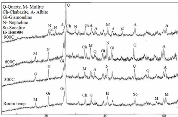
Fig. 8 X-ray diffractogram of GP8.5 specimen
