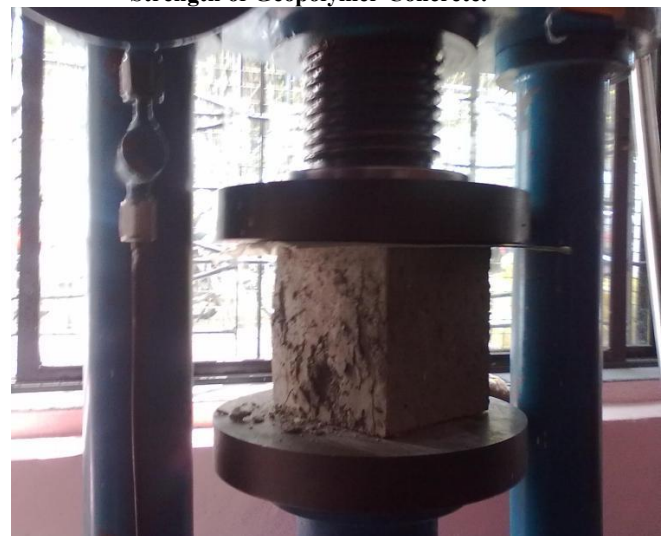
Fig. 3 Failure Pattern Of Fly Ash Based Geopolymer Concrete Cube In Compression Test.
