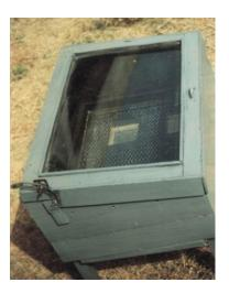
Figure 1 Picture of a direct passive solar dryer
