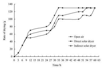
Figure 4 Drying rate curve for Pepper sample
