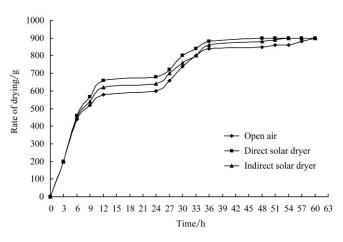
Figure 7 Drying rate curve for okro sample
