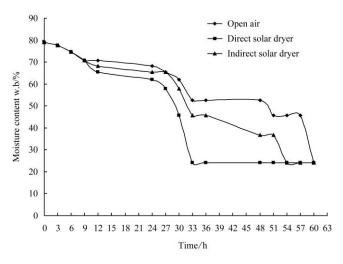
Figure 3 Solar dryer drying curve for pepper sample
