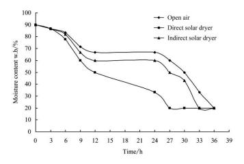
Figure 8 Solar dryer drying curve for vegetable sample
