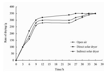
Figure 9 Drying rate curve for vegetable sample
