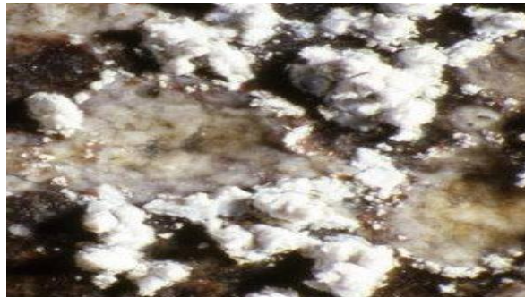
Corrosion of an engraved lead plate exhibited in an oak showcase
