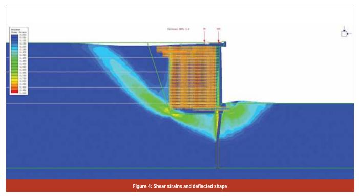
By tweaking the number and layout of piles, the deflections of the various components of the system were reduced to acceptable limits such that the differential settlements between elements were minimal
