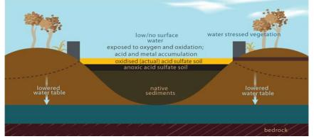
1.2 Exposure and oxidisation of ASS in a drying scenario (not to scale)
