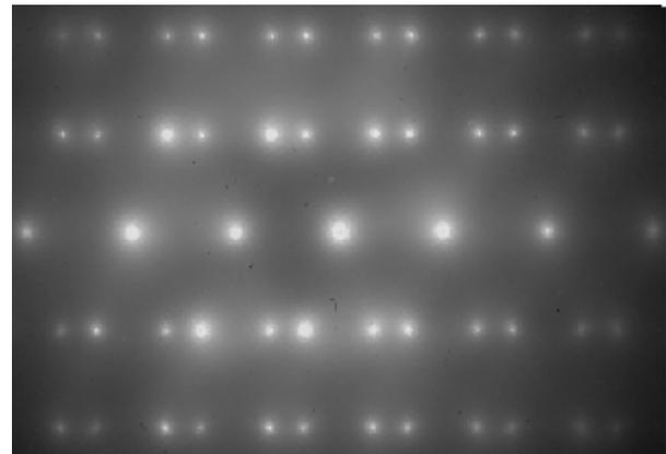
Diffraction pattern from nitrided surface layer of austenitic stainless steel
